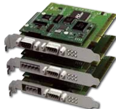
Fieldbus versions of the Anybus-PCI card built on standard Anybus technology
